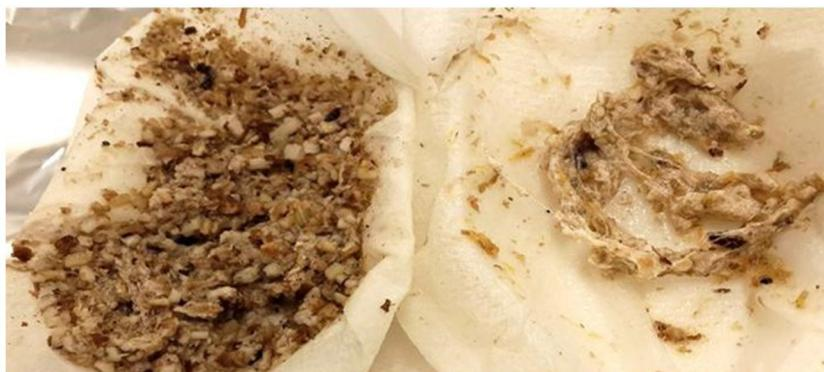
**Fig. 3.** Rubber produced by treatment of *Taraxacum kok-saghyz* roots with: (left panel) crude enzymes produced using wheat straw; (right panel) crude enzymes produced using guayule bagasse.
