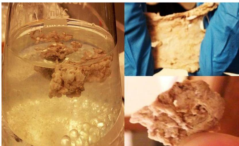
**Fig. 4.** Natural rubber extracted from *Taraxacum kok-saghyz* roots by growing *Thermomyces lanuginosus* STm on hydrolyzed root bagasse. Left panel: washed rubber in flask; upper right panel: rubber from flask lightly stretched indicating low contamination with plant material; lower right panel: unstretched rubber.
